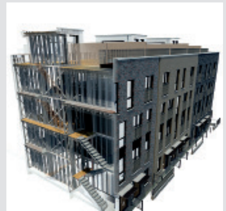
BIM model with 'warm frame' construction
