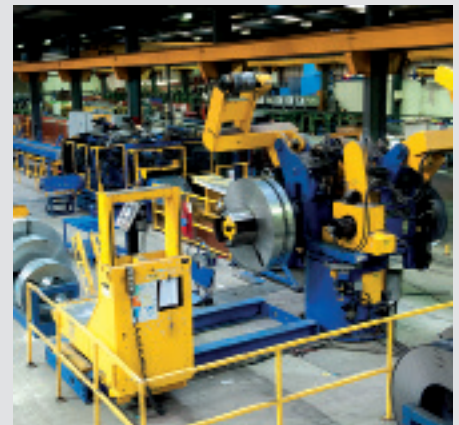
Components manufactured using automated roll-forming machines
