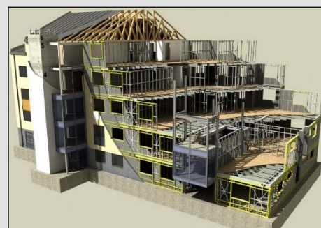
View of the Fusion framing system used in a 5 storey block
